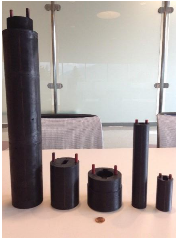
Figure 1.1: Scalable Fuel Grains Possible through Additive Manufacturing
