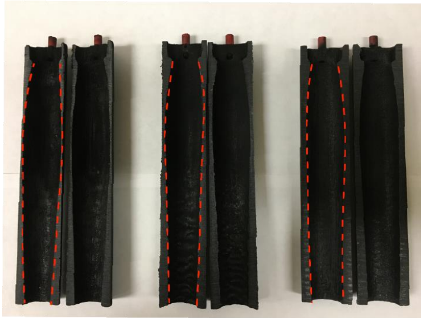
Figure 2.7: Fuel Port Bowing Effect in Samples of Burned Fuel Cells
