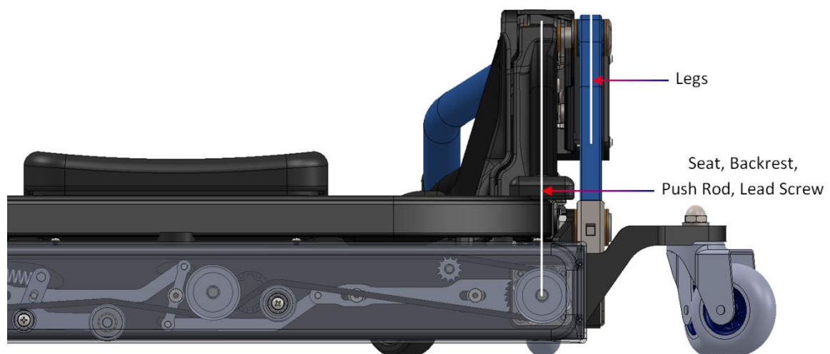
Figure 4: 3D kinematic link stacking of the Creep-Up creeper, showing how the respective links of the 2D kinematic chain are layered
