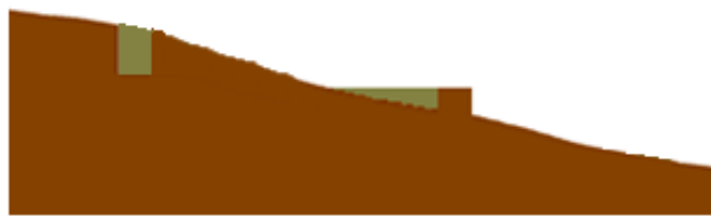
Pit Removal (Filling)
