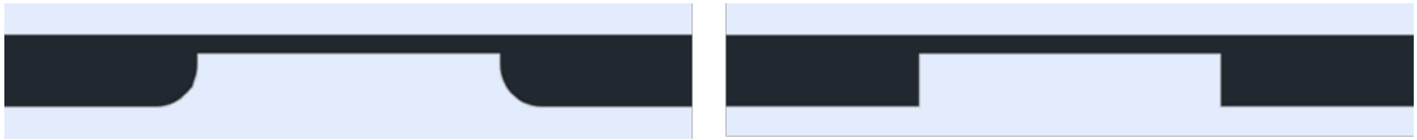
Figure 3: Examples of iDEP devices with partial obstruction. Illustrations are of a side view where the sample indicated by the dark grey color moves from left to right.
