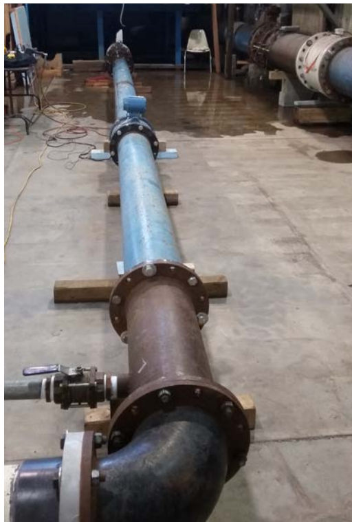
Figure 8. Phase II Straight Pipe Test Setup (flow top to bottom)
