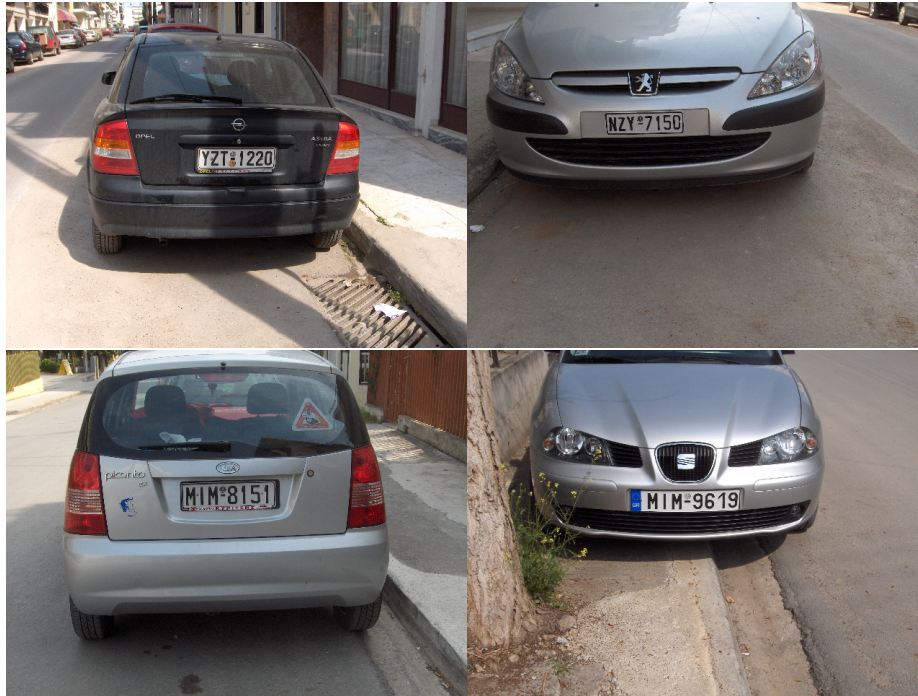
Fig. 3.1: Samples from the set of license plate images. The plates have different dimensions than American license plates, but the vertical edge densities are similar.
