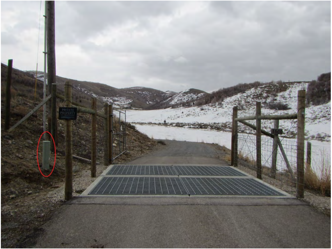
Figure 7. Motion activated wildlife camera (circled) used to monitor wildlife approaches to a wildlife guard on an access road to U.S. Highway 91, near Mantua, Utah, USA.
