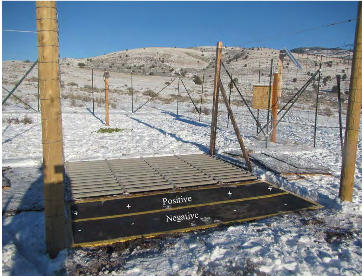
Figure 11. Close view of a 10 × 10-m wildlife enclosure used to test efficacy of 3 × 2.1-m cattle guards augmented with either 3 × 1.2-m (n = 2; pictured) or 3 × 0.91-m (n = 2) electrified pavement as an ungulate barrier at Hardware Ranch Wildlife Management Area, Utah, from mid-Oct 2014 to mid-March 2015. Positive and negative symbols added to indicate polarity of electrified pavement.
