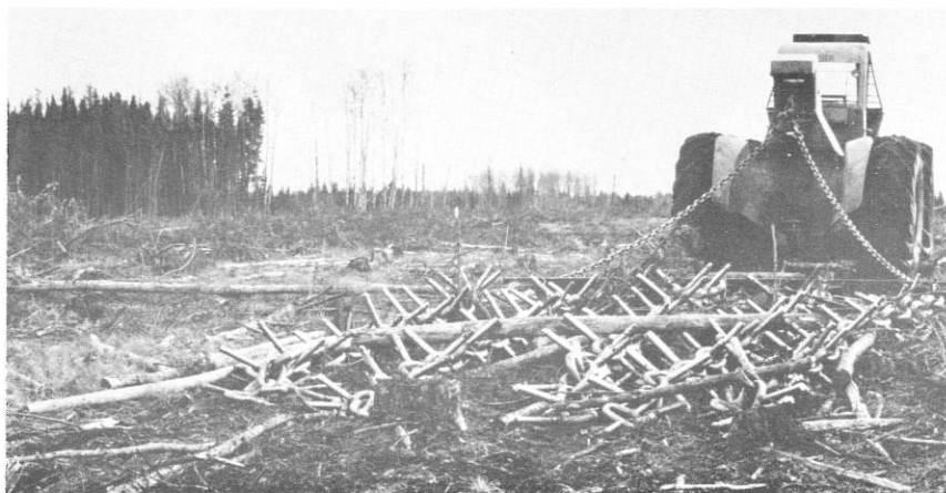
Anchor chains have become the principal scarifying tool in northern Manitoba.
