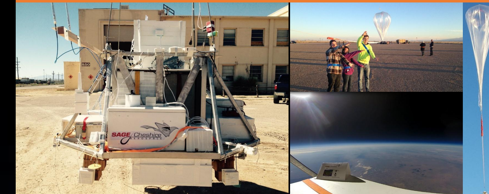
Fig. 9 Sage Cheshire high altitude balloon launch. Successful operation of OPTI in near space environment (no laser or time transfer test was performed, CSAC clock cycles counted).
