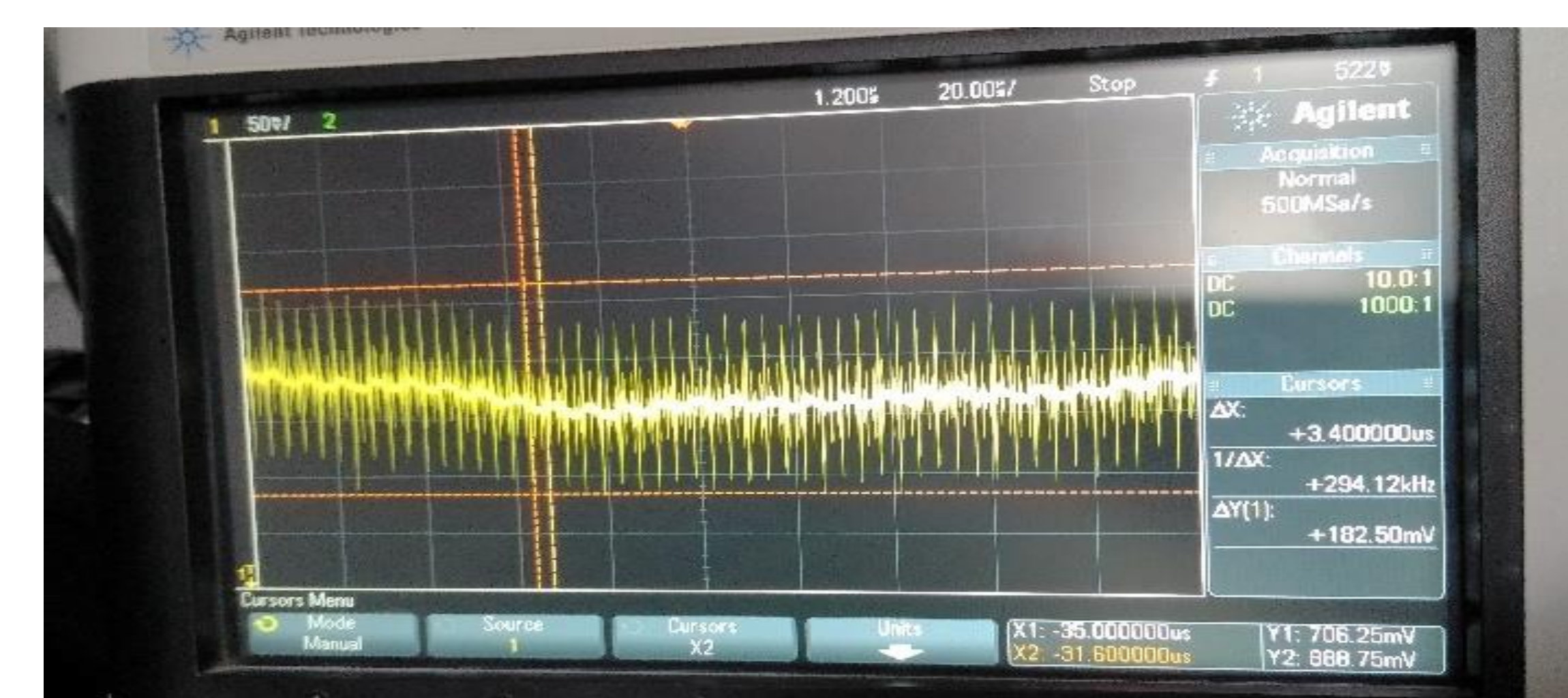
Fig 3 High Voltage Output before implementing filter design Scale : y axis -50 mV ; x axis -20 \mu s
