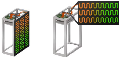
Figure 1: Left: Stowed Radiator System, Right: Deployed System.
