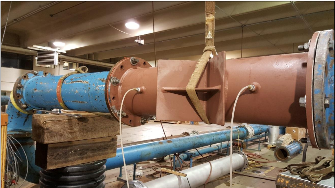
Figure 6: Horizontal or Out-of-Plane Installation of Wedge Flowmeter
