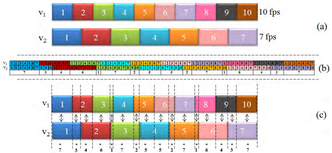
Figure 5.4. An example that shows how FRM compares two videos that have different frame rates.
