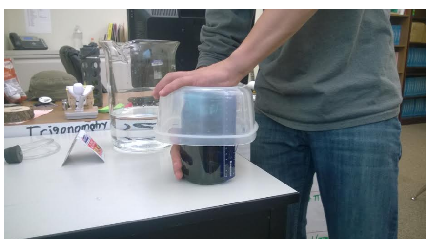
Figure 3: When flipping the container be sure to apply a fair amount of pressure on the plastic container to eliminate spillage.
