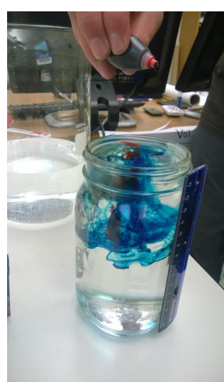
Figure 2: Food coloring is added to the water to help with seeing the height of the water when viewing the recording.
