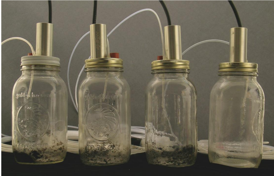
Figure 1: 1 liter Mason jars fitted with septa and oxygen sensors for gas measurements.
