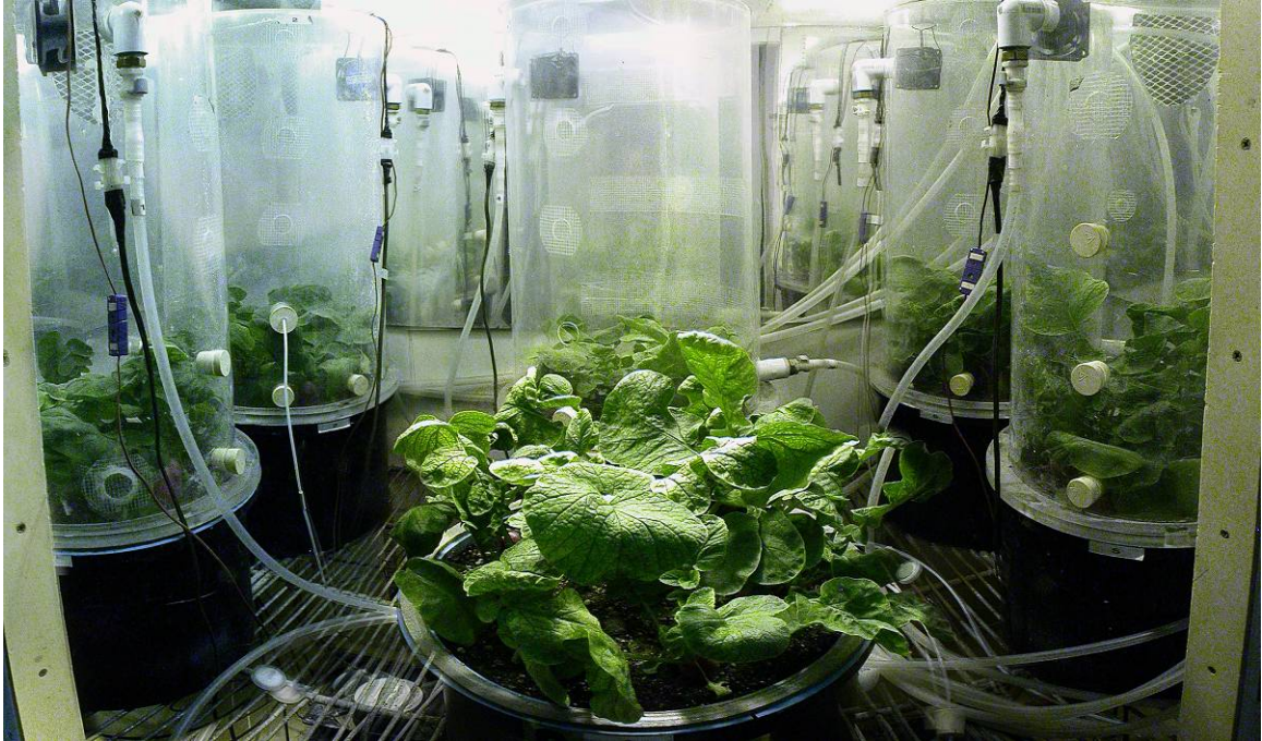
Figure 2-1. Example of radish plants in pots used for radish sensitivity and both PPF interaction trials. The front-center polycarbonate chamber has been removed for the photo. Blended-gas supply lines feed into the top of chamber directly in front of fan. Photo has been color corrected to remove orange cast of HPS lamps.
