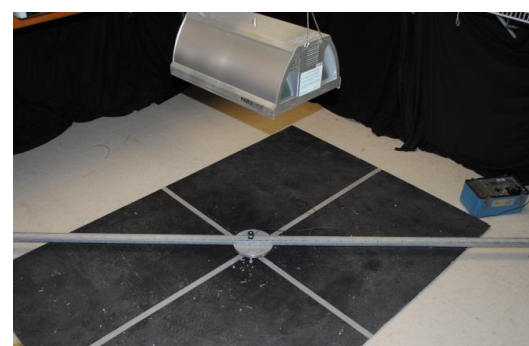
Figure 5. Set up for integrated total PPF measurement. Measurements must be made in a room without light contamination.
