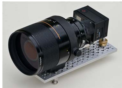
Fig. 5. COTS telescope and camera in ground-test configuration.
