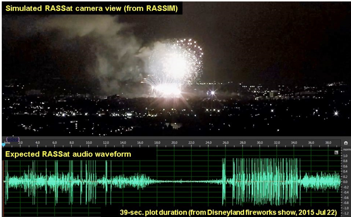
Fig. 3. Fireworks are a very strong opto-acoustic emitter and should be easily detectable in LEO by RASSat. This image shows the expected on-orbit visual and aural results for the proposed RASSat using the baseline sensors. Imagery was acquired from a 16-km (10-mile) distance using a 25-mm f/8 lens on a modified GoPro 4B camera and a 25-mm f/16 lens on the RAS detector.
