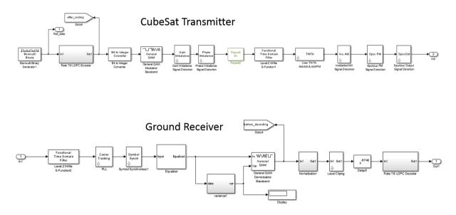
Figure 9: MATLAB®/SIMLINK Transmitter/Receiver Model Example
