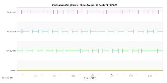
Figure 7: TDRS Daily Coverage for CubeSat at 500 km Altitude
