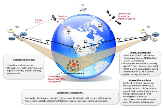
Figure 3: SN and NEN Supports both Single CubeSats and CubeSat Constellations
