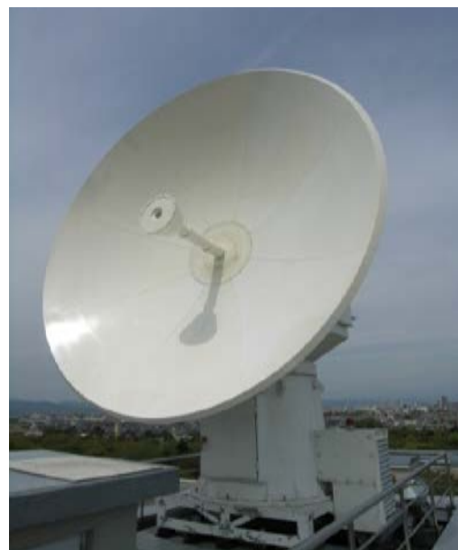
Fig.5: S/X dual band 3.8 m antenna at Sagamihara campus of ISAS/JAXA.
