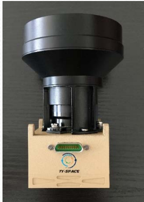
Nano star tracker (with baffle)
