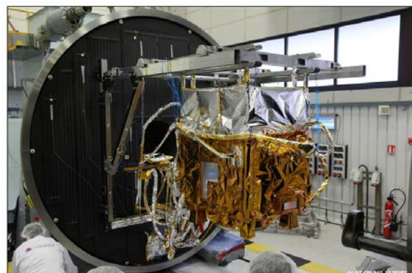
Figure 16: Satellite thermal vacuum test
