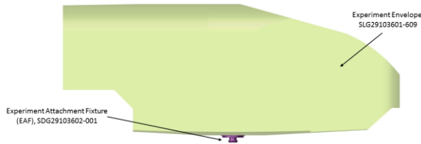
Figure 10: Cyclops Experiment Envelope
