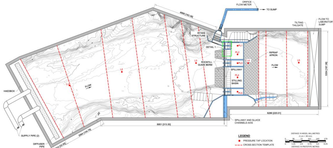
Figure 4. Plan view of the physical model.
