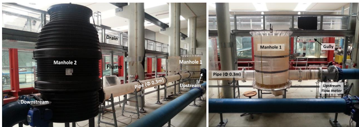
Figure 1: Multi-Link-Element experimental model setup at the hydraulic lab of the University of Coimbra
