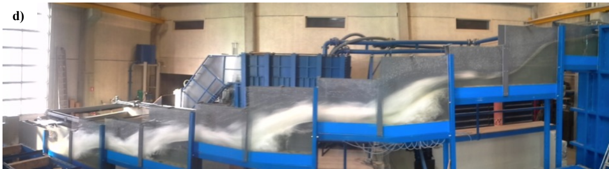
Figure 3. General view of the model – Prototype discharge of a) 25 m 3 /s, b) 50 m 3 /s, c) 75 m 3 /s and d) 100 m 3 /s
