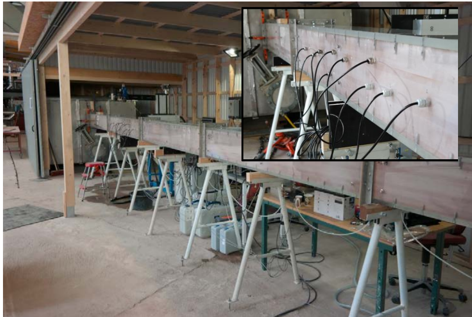
Figure 2. The rough surface channel; the pressure gauges can be seen just upstream of the downstream tank
