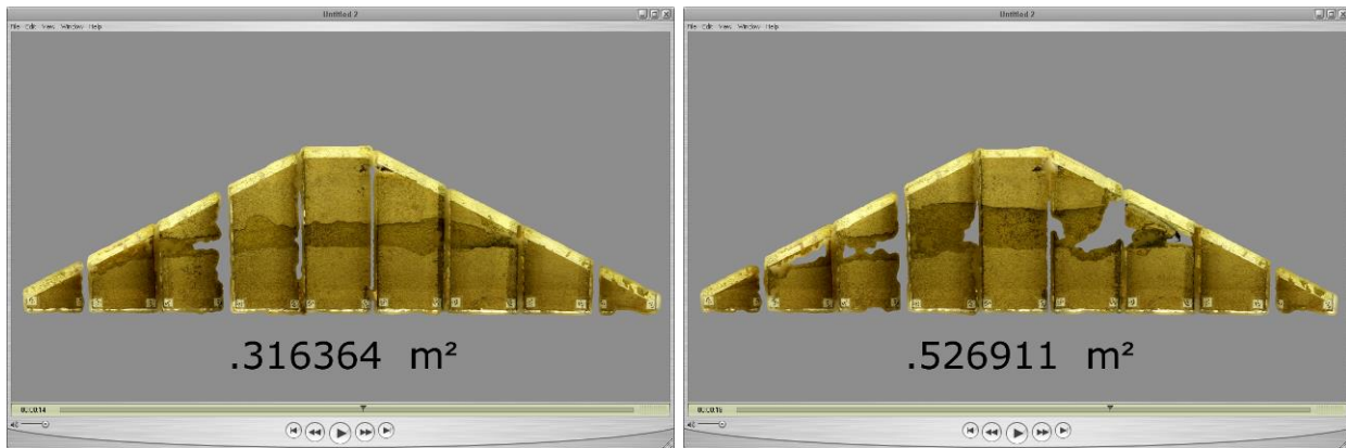
Figure 10. Two images from the 4D photogrammetry model of the internal erosion flow channel. In gray areas the model was not able to resolve the far side of the channel due to turbidity or other image quality problems.
