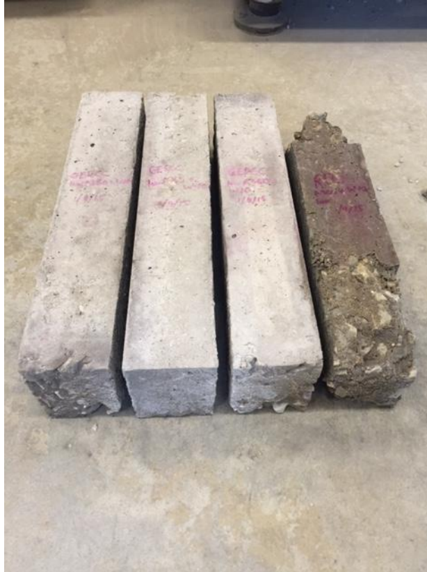
Figure 6. Freeze Thaw Samples After 300 Cycles
