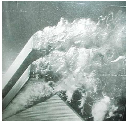
Figure 4. Cavitation Created in Low Ambient Pressure Chamber
