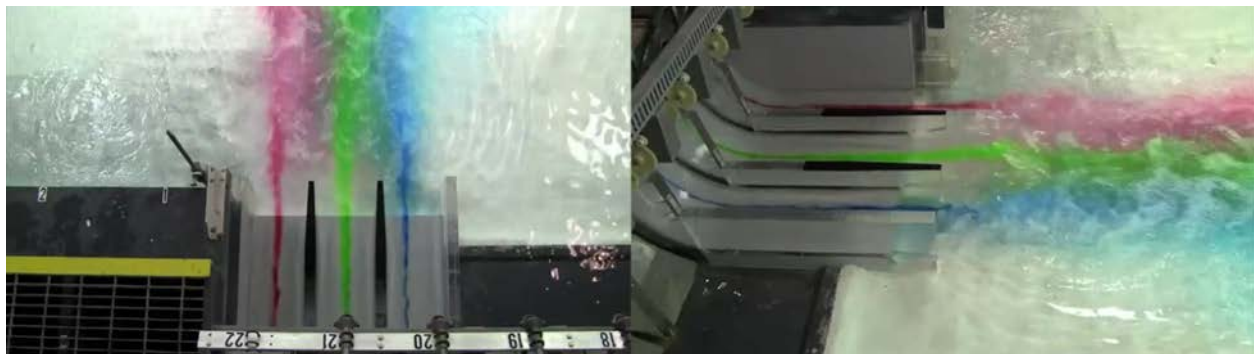
Figure 6. Fish bypass apron design being tested on the tailrace model.
