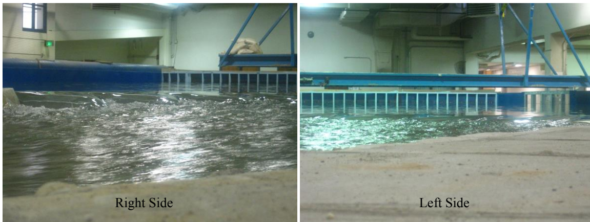
Figure 9. Submerged Weir (Baseline Design Configuration)
