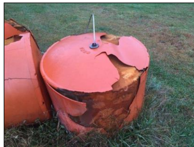
Figure 5: Degraded rotational molded boom. Photo: Andrew Peters, Pacific Netting Products
