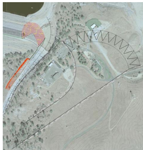
Figure 2. Proposed Spillway Configuration for Isabella Dam
