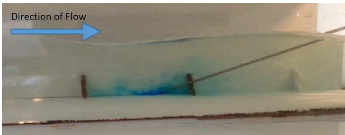
Figure 3. Photographs of slow flow and recirculation regions in the culvert barrel highlighted using dye injection - Flow direction from left to right
