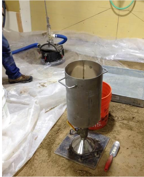
Figure 2. Sand cone (foreground) and submerged jet erosion tests (back, left) underway during a pause in embankment construction.
