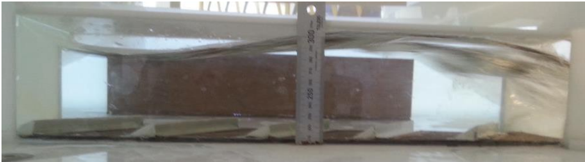
(A) Un-drowned barrel flow conditions for Q = 0.012 \text{ m}^3/\text{s} , \Delta h = 0.126 \text{ m}
