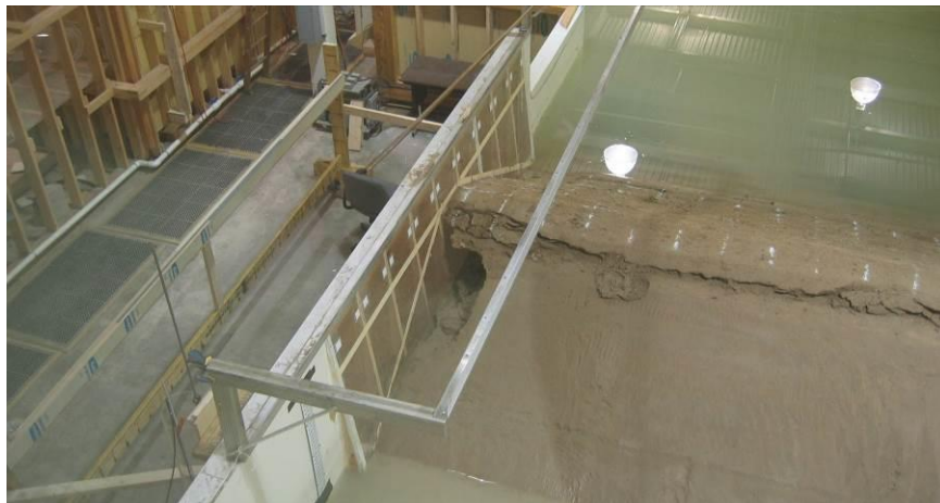
Figure 8. Post-test overhead view of the entrance to the internal erosion flow channel.
