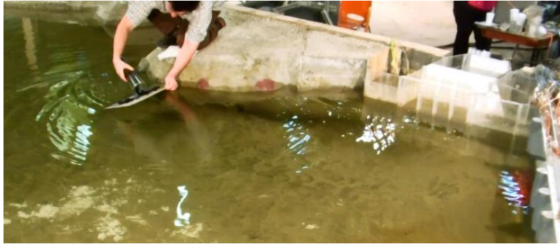
Figure 6. Photo showing injection of sediment upstream of the intake.
