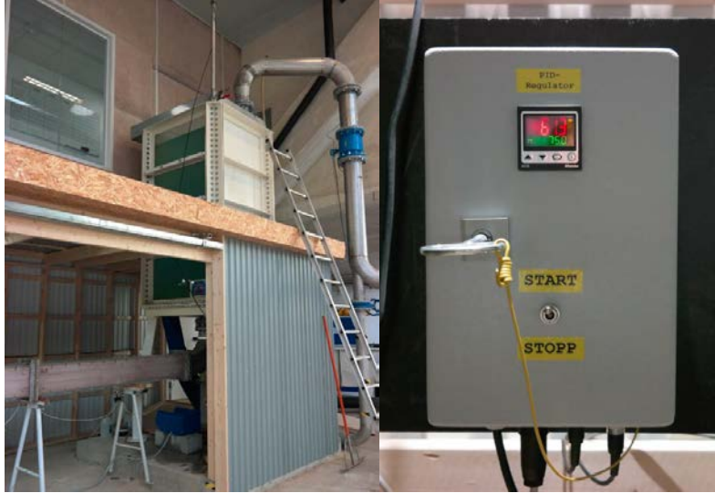
Figure 3. The upstream water tank and PID-regulator
