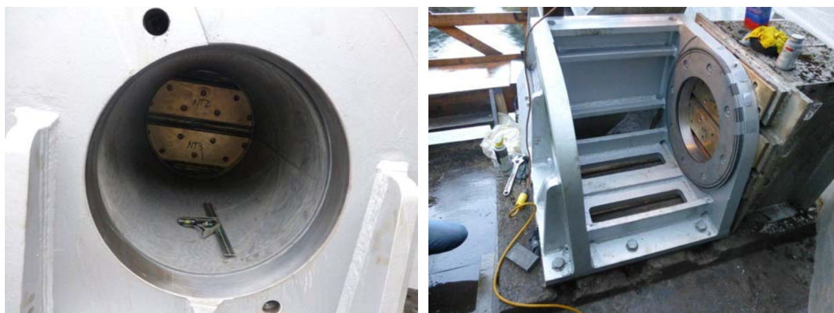
Figure 5. Self-Lubricated Trunnion Bearing and Thrust Washer.
