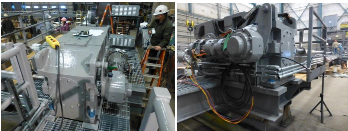
Figure 4. Shop Assembly and Testing of Skid Mounted Hoists.
