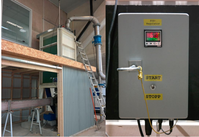
Figure 3. The upstream water tank and PID-regulator
