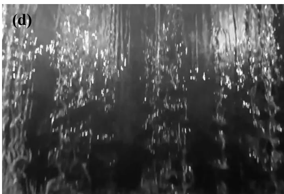
Figure 3. Nappe vibration visualization and associated Fourier transform of sound recording for (a) 0.015 \text{ m}^2/\text{s} , (b) 0.03 \text{ m}^2/\text{s} , (c) 0.045 \text{ m}^2/\text{s} and (d) 0.06 \text{ m}^2/\text{s}
