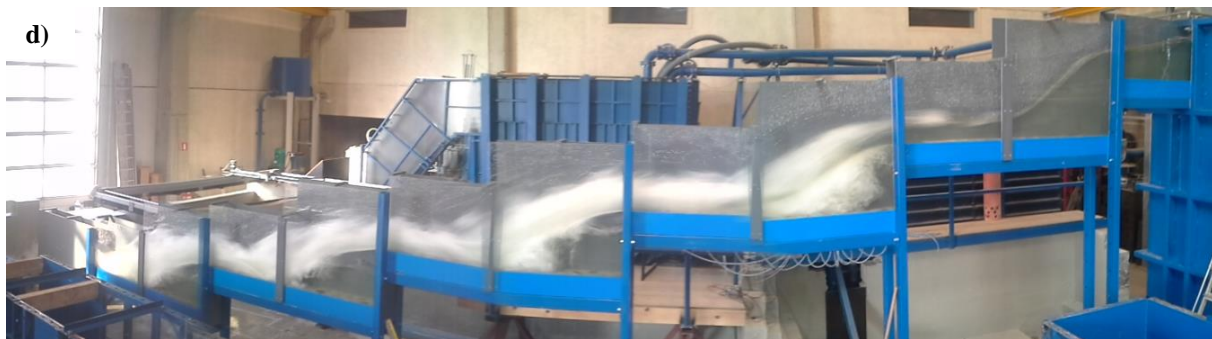
Figure 3. General view of the model – Prototype discharge of a) 25 m 3 /s, b) 50 m 3 /s, c) 75 m 3 /s and d) 100 m 3 /s
