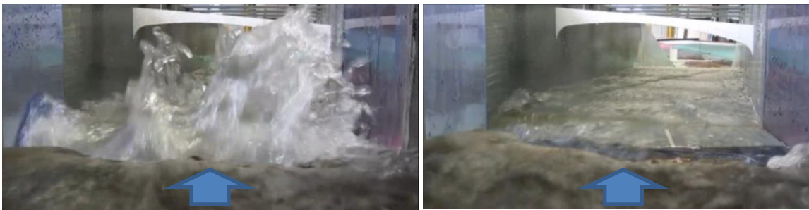
Figure 6. Comparison of the splashing effect in experiment series 4 and 5 (optimized geometry), Q = 100 \text{ m}^3/\text{s}
