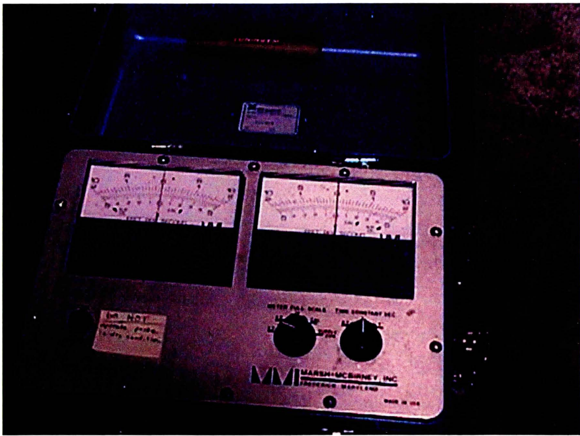
Figure A-C8 Marsh McBirney flow meter output display.
