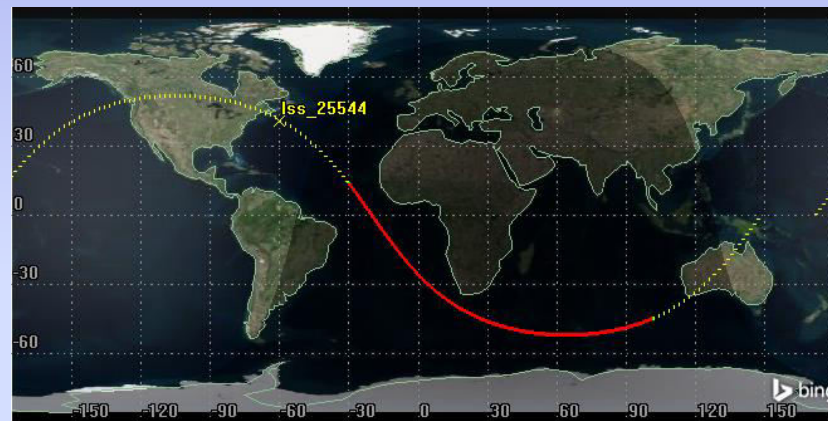
2-D map of the OPAL model with Yellow representing sunlit regions, and red in the umbra regions.
