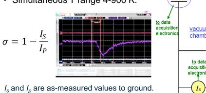
$I_{\rm s}$  and  $I_{\rm p}$  are as-measured values to ground  $\sigma \pm 0.005 \quad E_{max} \pm 1 \text{ eV} \quad E_{1} \pm 0.1 \text{ eV}$
