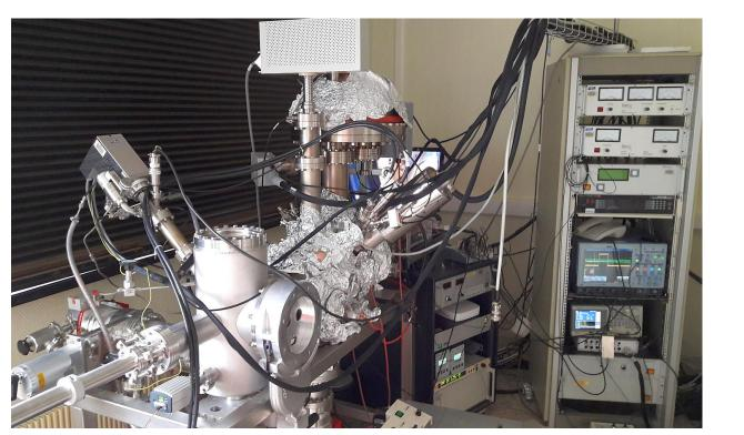
Electron emission yield was measured using the sample current method:
