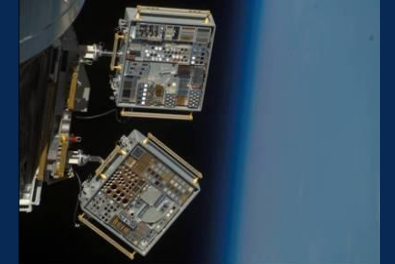
Figure 7 – MISSE, materials mounted to the ISS for long duration in flight radiation tests. Samples were characterized before and after flight.
