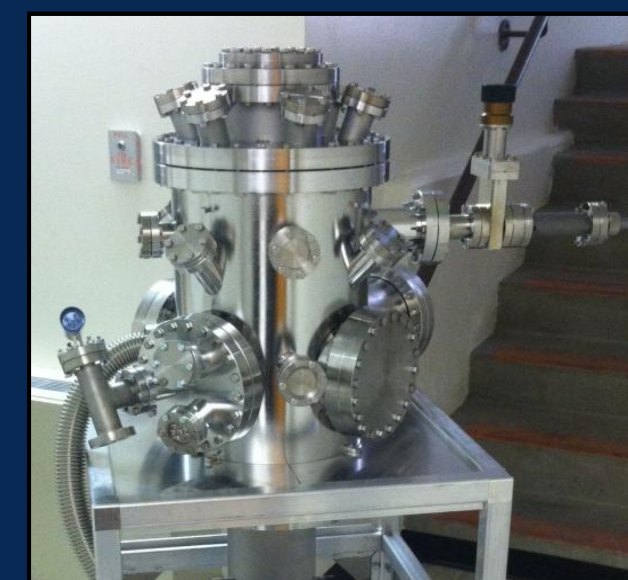
Figure 2 – The Space Survivability Test Chamber used to simulate the space environment in a controlled ground-based setting.
