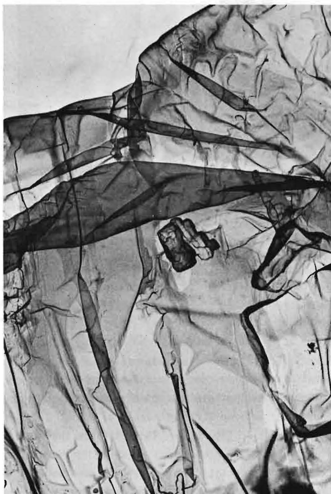
Figure 13. Electron micrograph of platinated surface replica of unreacted calcite single crystal surfaces at 18,000 x.
