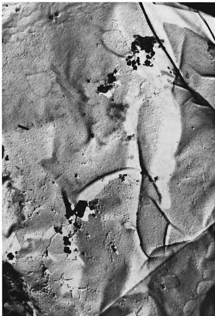
Figure 14. Electron micrograph of platinumized surface replica of calcite single crystal surface after reaction with phosphorus at 18,000 x.
