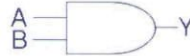
Figure 2. This circuit shows Boolean logic for an AND gate. If S1 (input A) AND S2 (input B) are closed, then the LED (output Y) will light. A circuit like this one is referred to as a Logic Gate.
