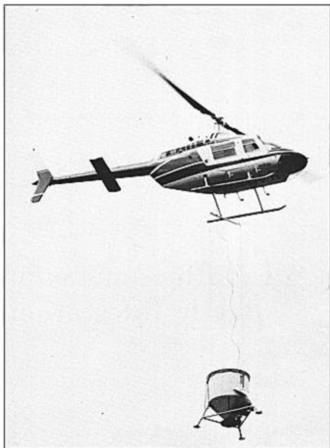
Figure 2. A modified aerial spreader and helicopter were used to apply granules containing pheromone.
