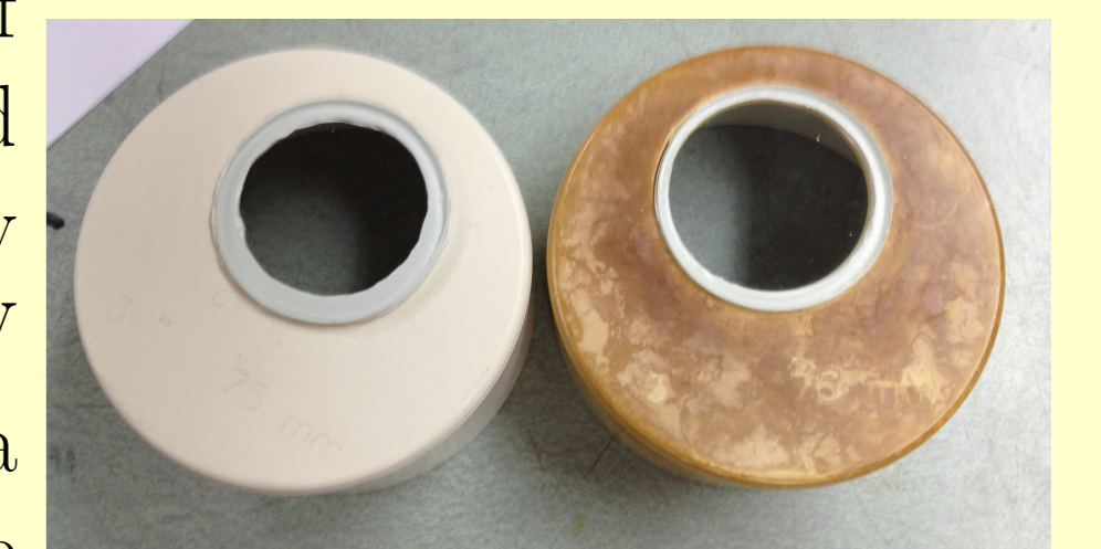
Figure 6: Two SQM-DL covers from different locations. The right cover was exposed to much more UV weathering, altering SQM readings.
