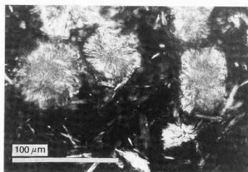
Fig. 1. Hydrogenated low erucic acid rapeseed oil as viewed under a polarized light microscope. Fat crystals ( \beta -polymorphic form) formed on spontaneous crystallization.
