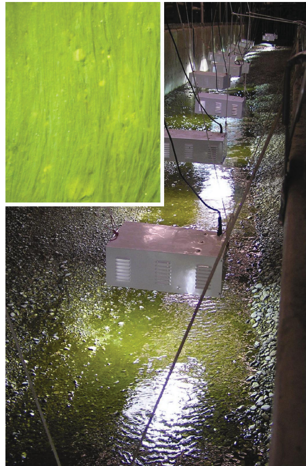
Figure 1. The St. Anthony Falls Laboratory Main Channel showing grow lights and periphyton growth during phase VI of StreamLab06. Inset is a close-up of a colony-forming river diatom ( Fragilaria spp.) that rapidly colonized the bed in response to light availability.
