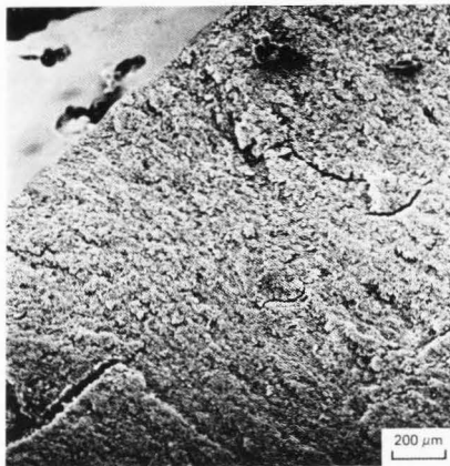
Fig. 7. Scanning electron micrograph of the concave fracture surface of a whey protein gel failed in tension.
