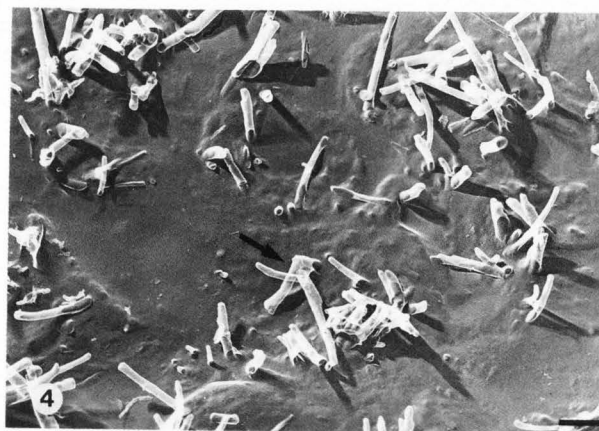
Figure 2. Form I Cocoa Butter, illustrating the lack of a distinct morphology. (Bar = 1 \mu m).
