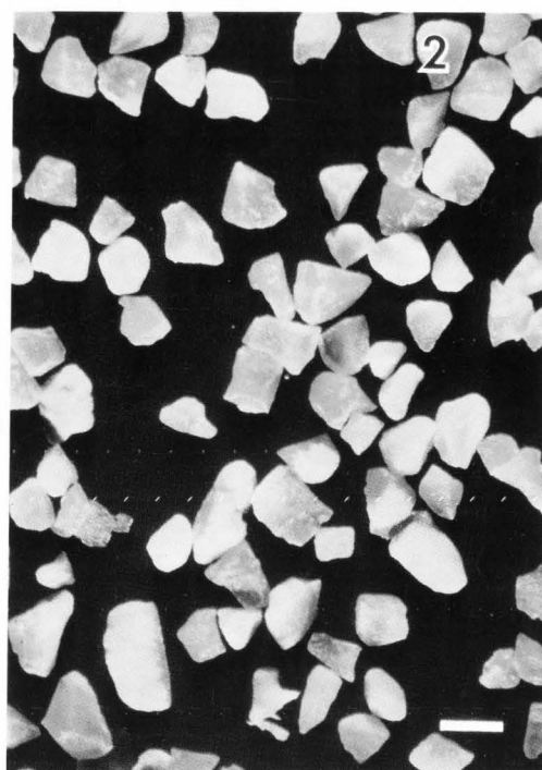
Fig. 2. Light micrograph of the coarse fraction (>0.710 mm) from Stenvert ground Bo Jac corn; bar = 650 \mu m.
