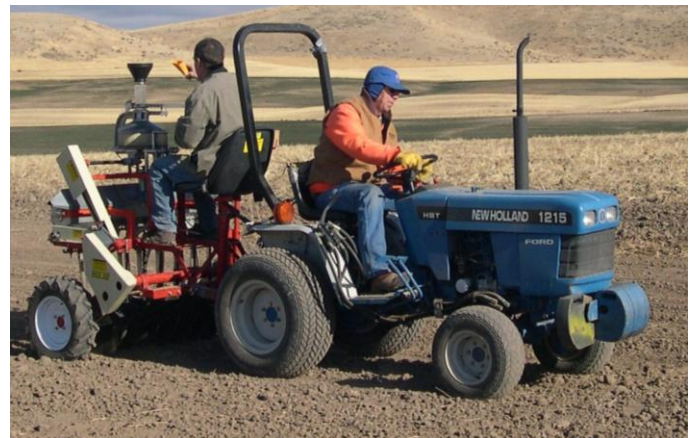
Figure 1. Planting safflower plots with a small-plot cone seeder.
