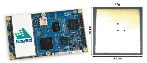
**Figure 7:** The NovAtel OEM628 GPS receiver is shown on the left, and one of the dual-band GPS patch antenna/LNAs is shown on the right. The GPSRO element of CTAGS (nominally zenith facing) consumes < 2W and the precision orbit determination element of CTAGS (nominally ram facing) consumes  $\sim 1.3W$ .
