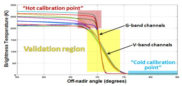
**Figure 2:** Representative brightness temperature as a function of scan angle near the Earth's limb for the MiRaTA channels. With knowledge of the atmospheric state, which will be provided with very high accuracy (~0.25K (Ho, Schreiner, & Zhou, Using SI-traceable Global Positioning System radio occultation measurements for climate monitoring, 2009)) by the GPSRO measurements, this distribution can be calculated to very high accuracy (~0.3K) by a limb-optimized radiative transfer model [6].
