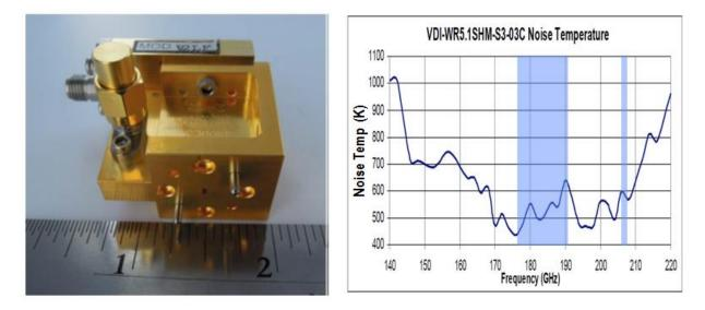
**Figure 5:** The Virginia Diodes, Inc. (VDI) wideband mixer front end will provide double-sideband measurements in three channels near the water vapor absorption band (183.31  $\pm$ 1,  $\pm$ 3, and  $\pm$ 7 GHz), and a single-sideband measurement of a 206.4 to 208.4 GHz cloud ice band.
