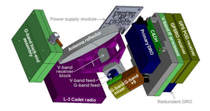
**Figure 6:** MiRaTA tri-band sounder (antenna shroud not shown) and GPS receiver notional layout. Total radiometer mass is 907g and power consumption is 5.5W. Assembly size is 10 x10 x18 cm.
