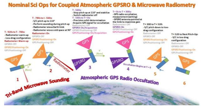
**Figure 3:** The MiRaTA primary mission validation concept of operations (ConOps) is shown above. A slow pitch maneuver ( $\sim 0.5^{\circ}$ /sec) is used to scan the radiometer fields of view through the Earth's limb and subsequently direct the CTAGS field of view through the same atmosphere to catch a setting occultation. The entire maneuver takes about 20 minutes and is performed once per orbit over a 60-day validation period (approximately 1000 total scans).
