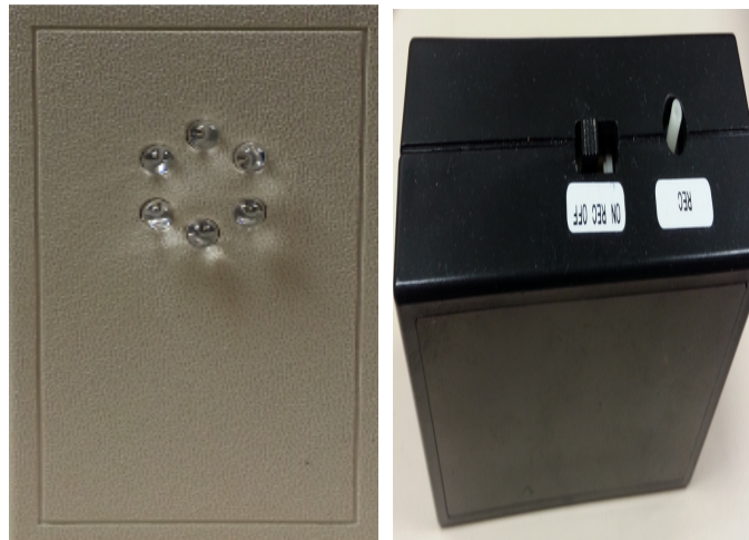
Figure 4.2 RIAS Transmitters fitted to aisles
