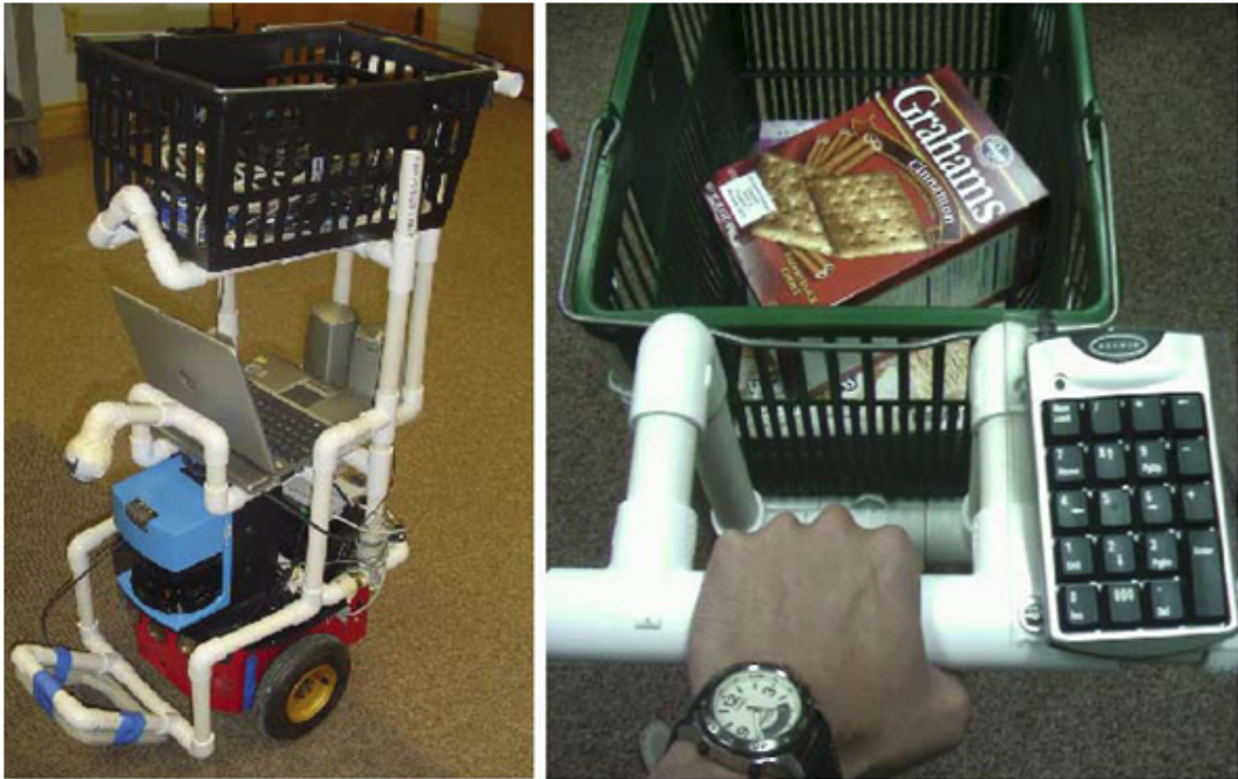
Figure 2.1 RoboCart (left); RoboCart's handle with Belkin 9-numeric keypad (right)
