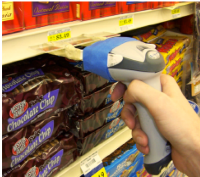
Figure 2.3 Barcode scanner with the added stabilizers, resting of a shelf lip
