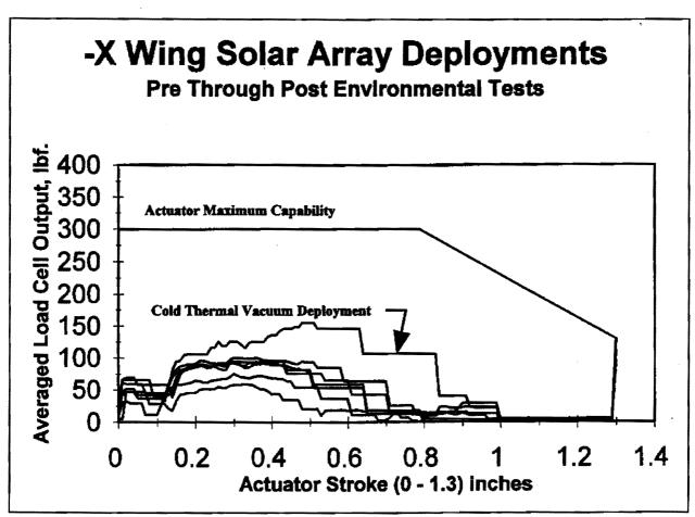
Figure 8, Composite Solar Array Deployments (-X Wing)
