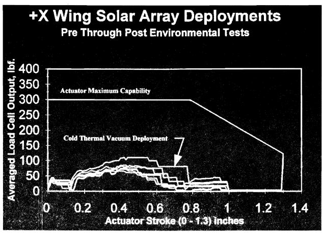
Figure 7, Composite Solar Array Deployments (+X Wing)
