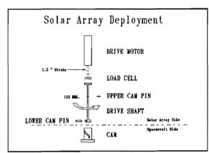
Figure 4, Mechanism Components
