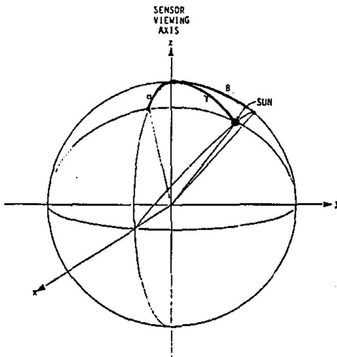
Figure 2. Sun's spherical coordinates in sensor's coordinate system
