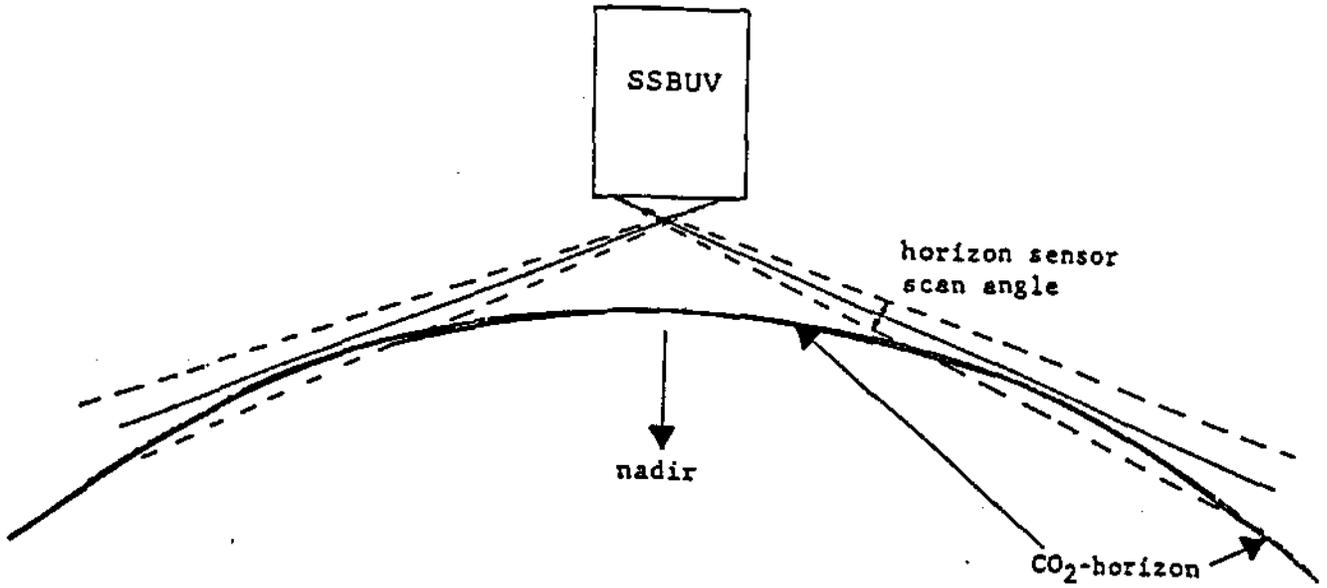
Figure 6. Aspect determination by a horizon sensor using a scanning mirror
