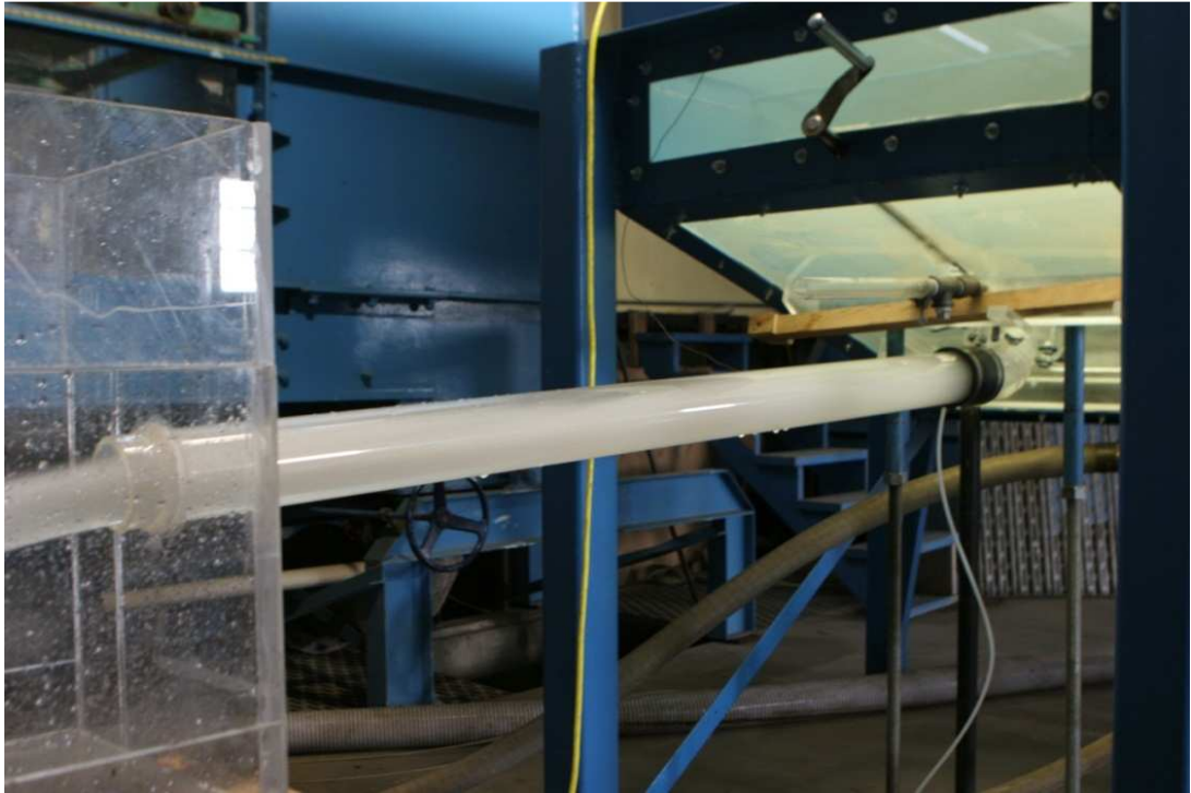
Figure 7: Low-level outlet works setup
