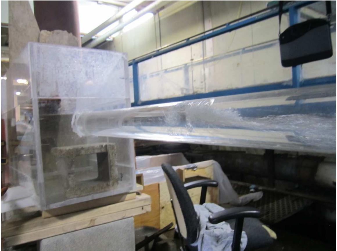
Figure 30: Hydraulic jump forming in the outlet works
