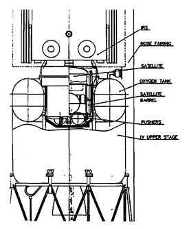
Figure 1. The Skipper satellite placed in the fourth stage of the Molnia launch vehicle.
