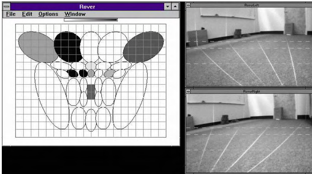
Figure 32. Images and map with left wheels elevated.
